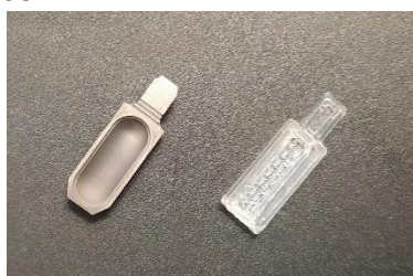
Fig 1. Original pyrolytic graphite platform (left) and 3D polymer platform (right).
